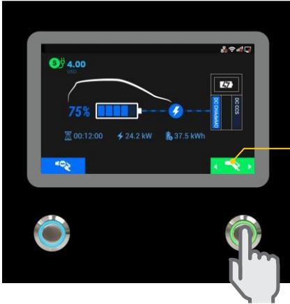
Press right button to select the charger connector that the user would like to stop.
