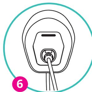
When BLUE LED is on, your **easyWallbox** is ready to be used in Plug & Play Mode (up to 2.3 kW)
