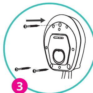
Take the **easyWallbox** (remove the aesthetic cover) and fix the 3 screws into the fixing plugs
