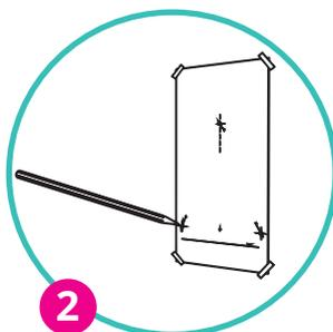
Using the drilling template, mark where to drill on the wall and insert the 3 fixing plugs into the holes
